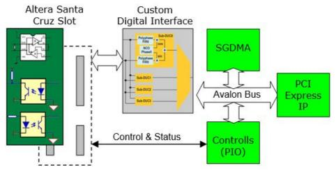
PCIe Fpga card allows an easy building of customized interfaces to be used on the PC, such as serial synchronous HDLC, RS422, RS485, optional high speed DMA:
