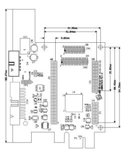
The fpga signals available on J1-J3 connectors are 3V3 tollearant.
