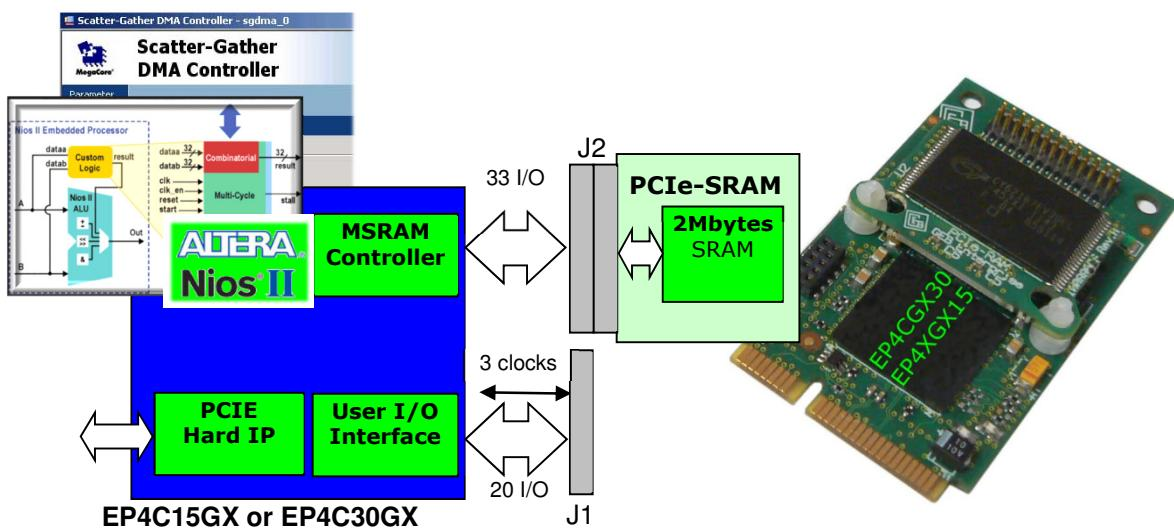
The NIOS micro controller make available to the developers the handling of I/O interrupts in few tens of ns with deterministic latency, customized instructions that will be able to process your data with a speed and a continuity that are most difficult to reach on the host CPU. Moreover the NIOS can implements a multi channels virtual DMA between lots of high & low speed I/O and the main memory.
