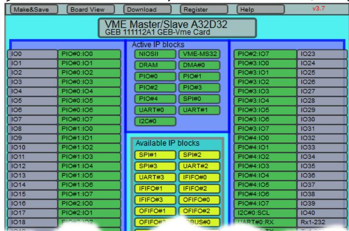
Different custom versions of external interface for specific application can be developed by GEB or by user, using Altera's tools, such as QuartusII and SOPC Builder or QSYS.
