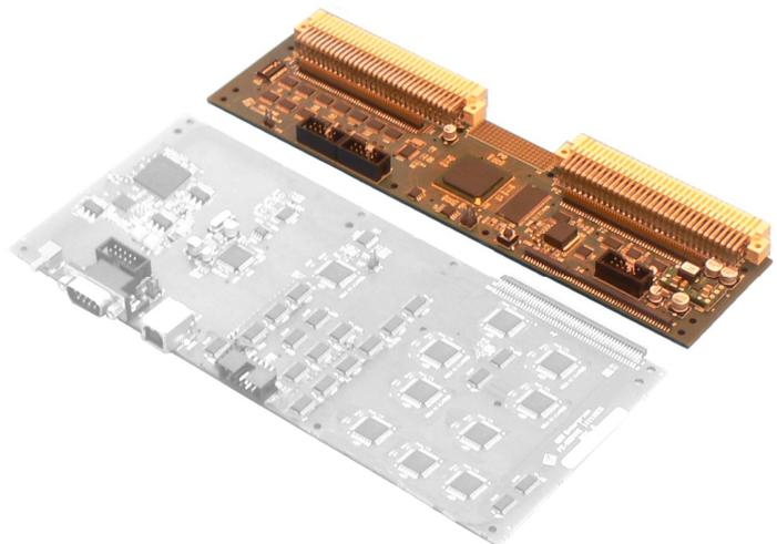
The current VME IP and NIOS firmware supports A32D32 master/slave cycles, interrupt handler, interrupter and SysCon. The related firmware (Monitor), running on NIOSII, allows the user to start all kind of buses cycles and some macro commands, such as memory test, using RS232 or USB data link.
