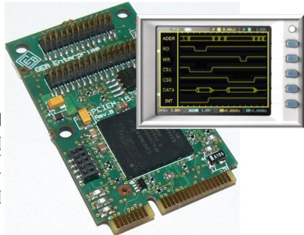
The IOBUS shall be the bus used for communication between a master (the PCIe card) and an unspecified number of slaves. The bus supports up to 32 Data bits, up to 8 bits address, 2 Chip Select (CS#), Read Enable (RD#), Write Strobe (WR#), Interrupt request (INT#) and an optional Wait signal (WAIT#).
